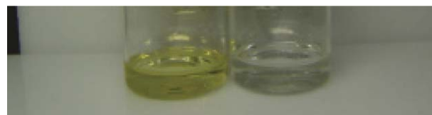
Fig. 1 Commercial quality 1-ethyl-3-methylimidazolium bis(trifluoromethanesulfonyl)amide (left) and a sample made in our laboratory (right).
